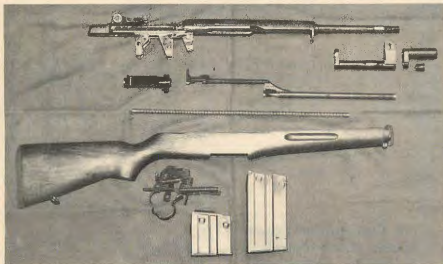
Beretta BM-62 7.62 NATO rifle field-stripped. Note simplicity of components. Ten and 20-round magazines at bottom.
